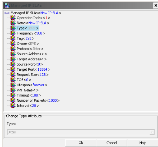
Figure 438 Configuring UDP Jitter Operations
