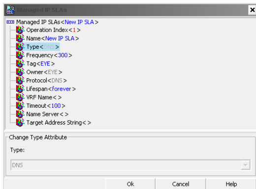
Figure 432 Configuring DNS Operations
