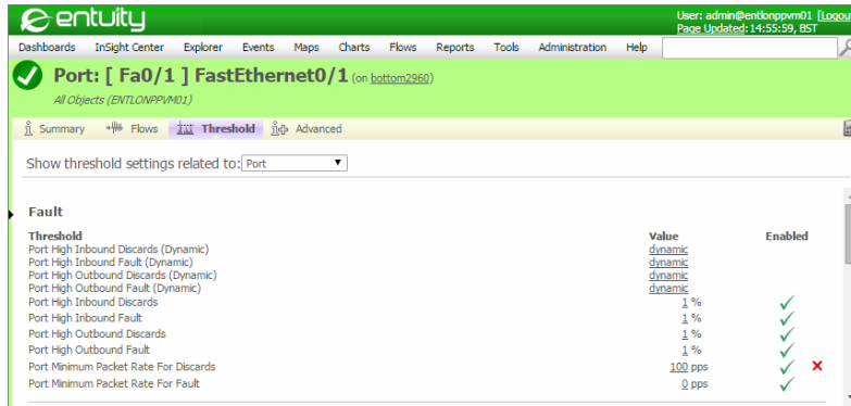
Figure 170 Thresholds for Minimum Packet Rate
